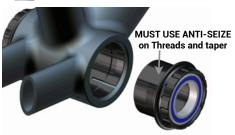
**4**. On the Drive Cup, put a thin coat of **ANTI-SEIZE** on the threads and on the taper smooth area just above the threads. Then start threading the Drive Cup in CLOCKWISE with your BB tool. As it threads in, you will feel friction build as the collet expands. This is when you grab your 2nd BB tool.
