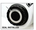
**6**. Dab some grease on the underside of the included seals, then place seals on the bearings with Praxis logo facing outward (larger metal surface outward.)
