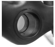
**3.** The Delrin PF cups need to be pressed in flush to the frame. Once you make sure the PF cups are flush, you're ready to install the Conversion BB.
